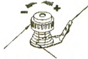
Threading the pre-tension for bobbin winding
